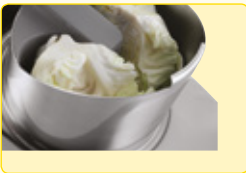
Round stainless-steel hopper (215 cm 2 )
